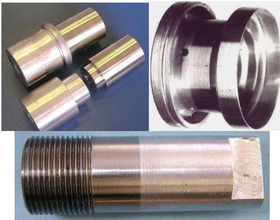
Fig. 1 – FW joints of aluminum alloy AMg6 to stainless steel using intermediate element of aluminum AD1 (components for fuel system of rocket engine)
